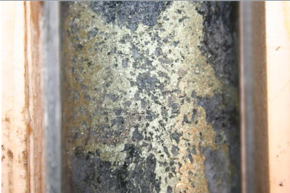
Sulphides in Falun drill core
