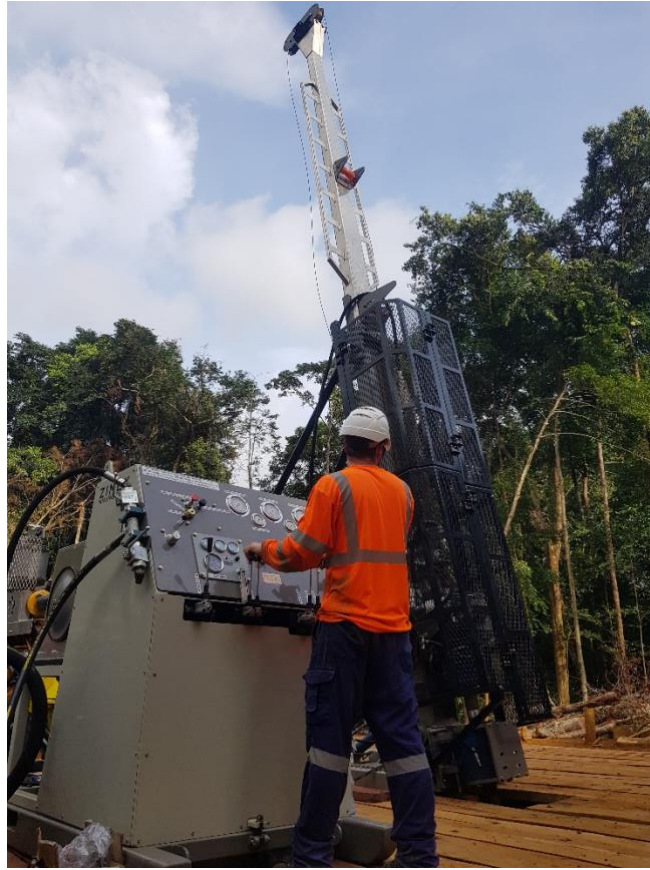
Figure 1: Custom-built Zinex A5 diamond drill rig set-up at the first drill hole site at Libonga North. Source: AMM.
