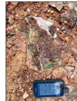
Outcropping copper-rich gossan and breccia observed at Kurili Hill Prospect.
