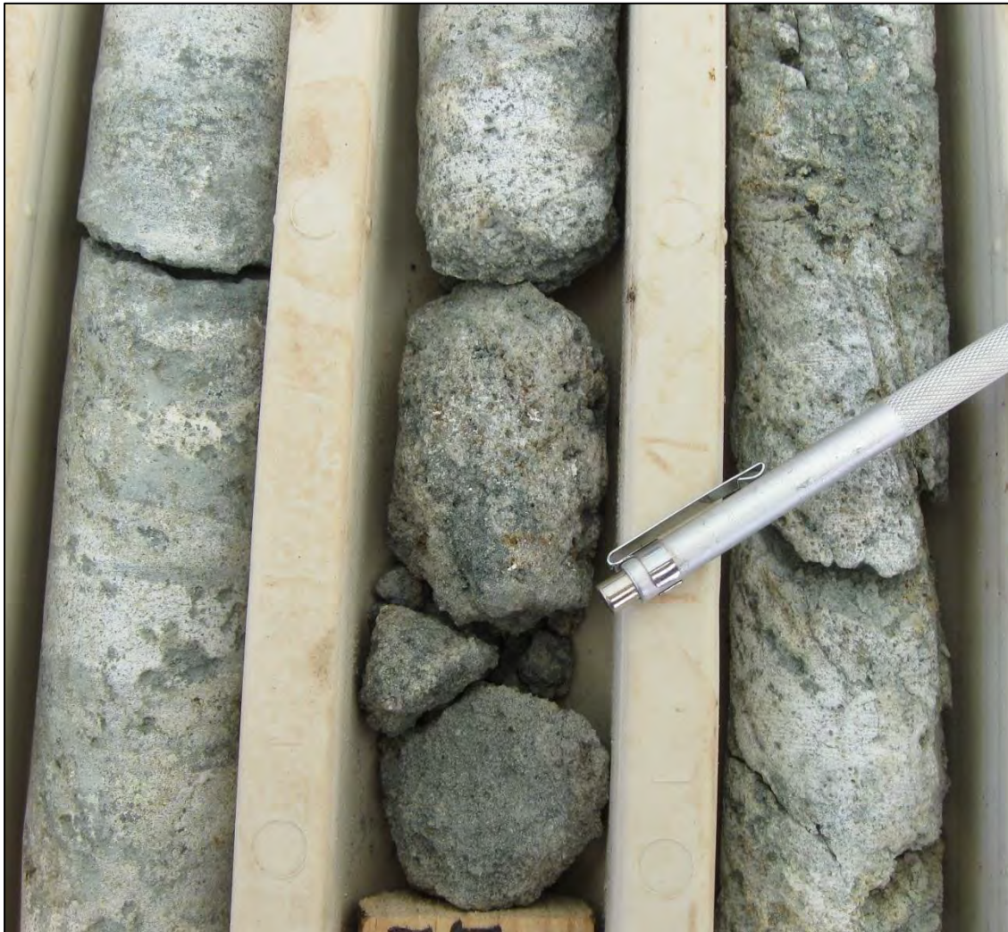
[Figure 5] Maronan Project: Typical strong visible lead sulphide mineralisation from fresh banded carbonate-lead sulphide rock in MRN12003B at 1234.3 metres down hole (above). The dominant grey-silver mineral is lead sulphide (galena). Strongly weathered and potentially leached banded carbonate rock with strong chlorite, weak to moderate lead oxides and minor relict lead sulphide from current hole MRN12004 (right at 834.3m and below at 845.1m). Is this material an oxidised, potentially leached, version of mineralisation in MRN12003B? Assay results from MRN12004 are pending.
