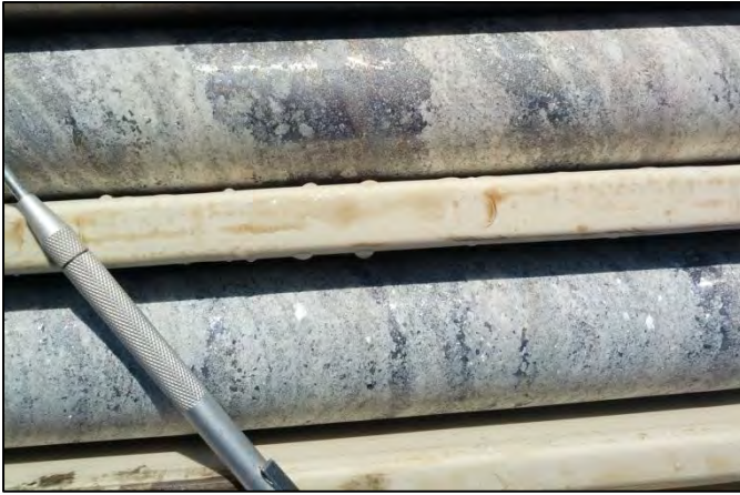
[Figure 5] Maronan Project: Typical strong visible lead sulphide mineralisation from fresh banded carbonate-lead sulphide rock in MRN12003B at 1234.3 metres down hole (above). The dominant grey-silver mineral is lead sulphide (galena). Strongly weathered and potentially leached banded carbonate rock with strong chlorite, weak to moderate lead oxides and minor relict lead sulphide from current hole MRN12004 (right at 834.3m and below at 845.1m). Is this material an oxidised, potentially leached, version of mineralisation in MRN12003B? Assay results from MRN12004 are pending.
