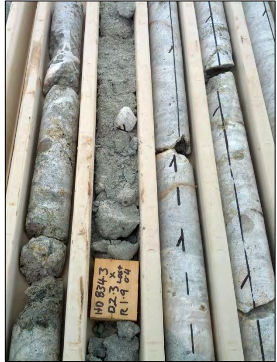
[Figure 5] Maronan Project: Typical strong visible lead sulphide mineralisation from fresh banded carbonate-lead sulphide rock in MRN12003B at 1234.3 metres down hole (above). The dominant grey-silver mineral is lead sulphide (galena). Strongly weathered and potentially leached banded carbonate rock with strong chlorite, weak to moderate lead oxides and minor relict lead sulphide from current hole MRN12004 (right at 834.3m and below at 845.1m). Is this material an oxidised, potentially leached, version of mineralisation in MRN12003B? Assay results from MRN12004 are pending.
