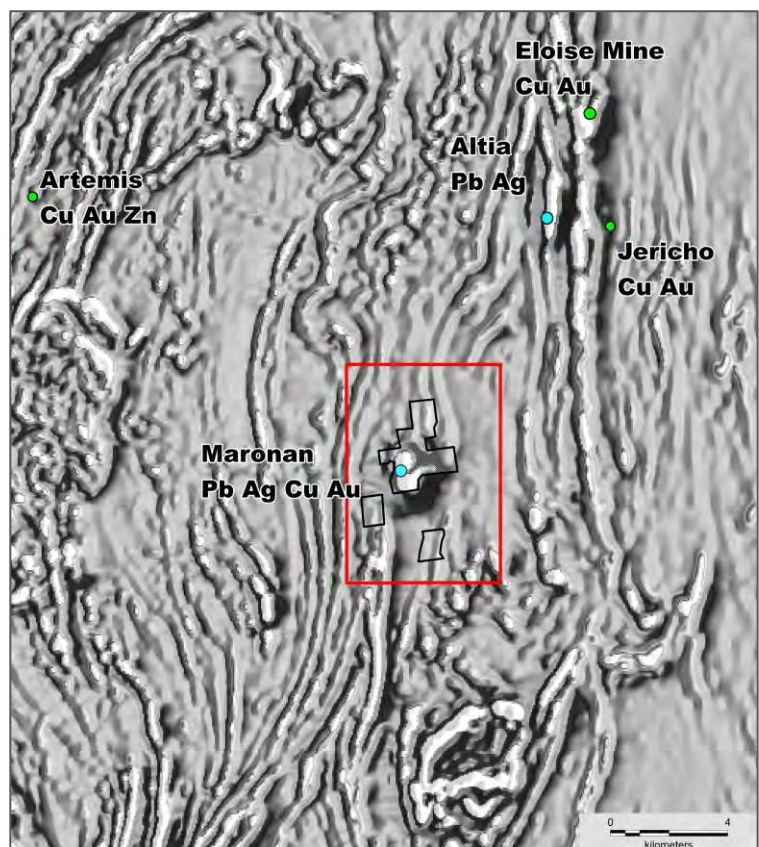
[Figure 1] Maronan Project: Regional vertical gradient magnetic image showing the Maronan lead-silver and copper-gold deposit, other copper-gold and lead-silver-zinc prospects and the Eloise mine. Historic ground electromagnetic survey grids on Maronan are shown as black polygons.
