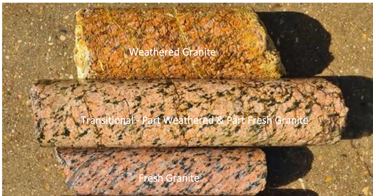
[Figure 4] Sybella Project: weathered, transitional and fresh REO-enriched granite (top). Note the coarse grain-size, weak biotite deformation fabric and increased fracture density with increased weathering.
