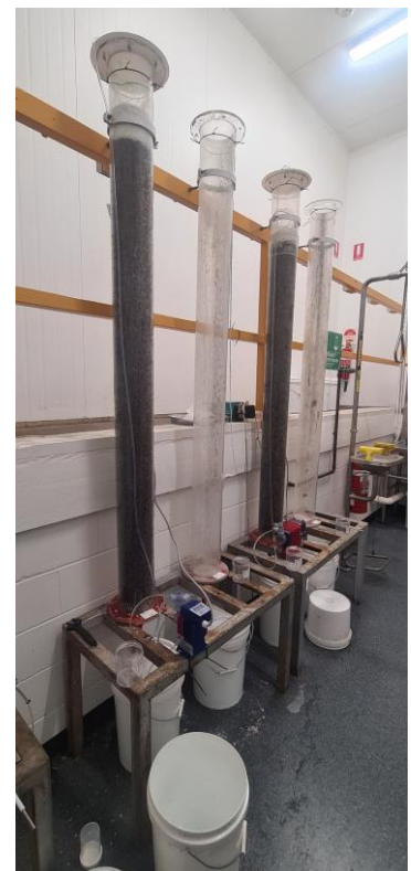
[Figure 12] Sybella Kary Zone: Intermittent bottle roll set-up (left) and an example of column leach test setup (right).
