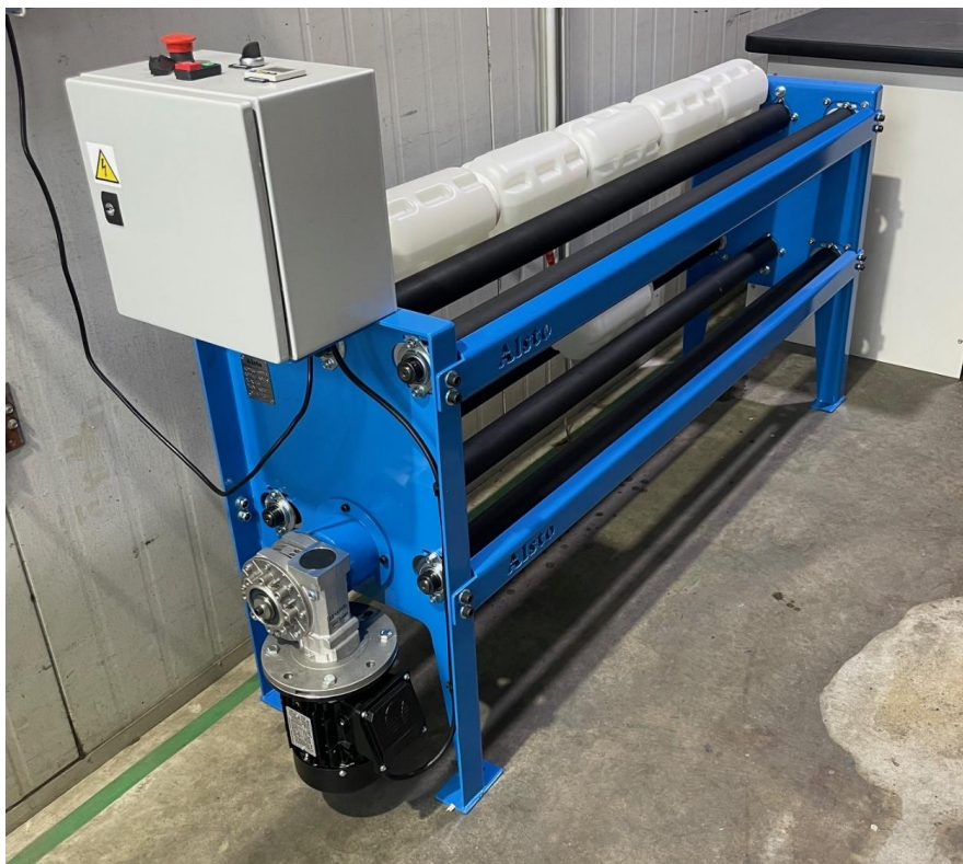
[Figure 12] Sybella Kary Zone: Intermittent bottle roll set-up (left) and an example of column leach test setup (right).
