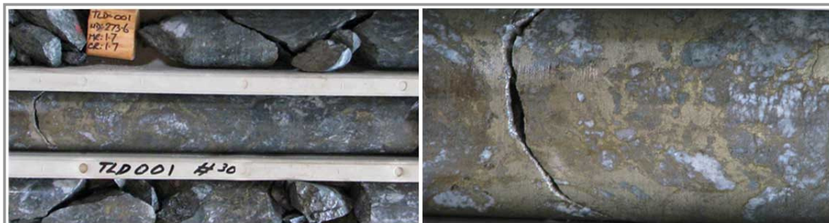
Panel 2. Eastern Zone diamond cores from TD1 (NQ - diameter 4.8cm) showing massive chalcopyrite (CuFeS 2 ) mineralisation.
