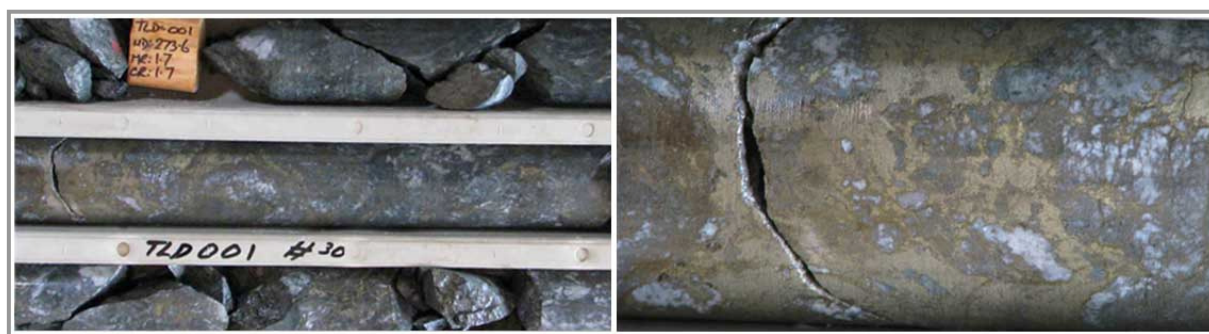
Panel 2. Eastern Zone diamond cores from TD1 (NQ - diameter 4.8cm) showing massive chalcopryrite (CuFeS 2 ) mineralisation.
