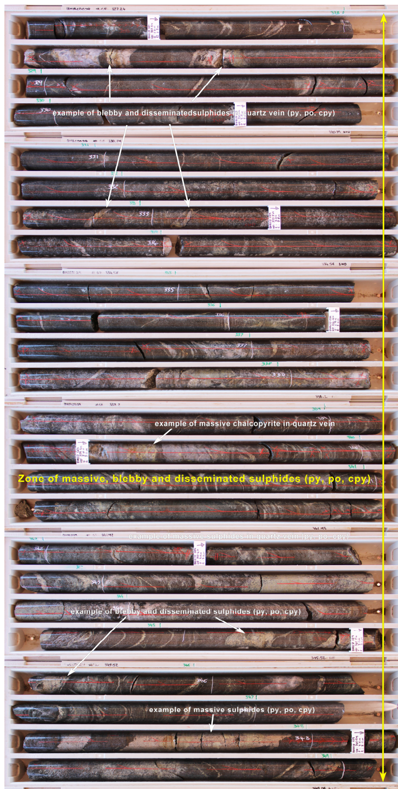
Figure 2: Drill core from 327.24 - 349.24m BHRCD029, showing massive, blebby and disseminated sulphides
