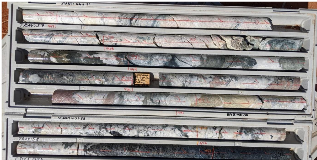
Figure 2 - Mineralised zone from 448.8m to 452.6m down-hole, with mineralised Monazite and Bastnasite in Carbonatite, confirmed with pXRF analysis
