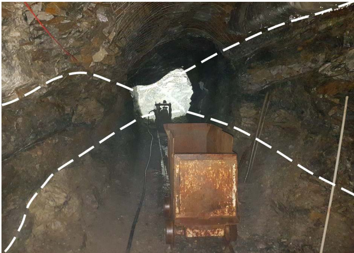
Figure 1 – 10 MLS drive with the mineralised envelope shown as the white dashed line
