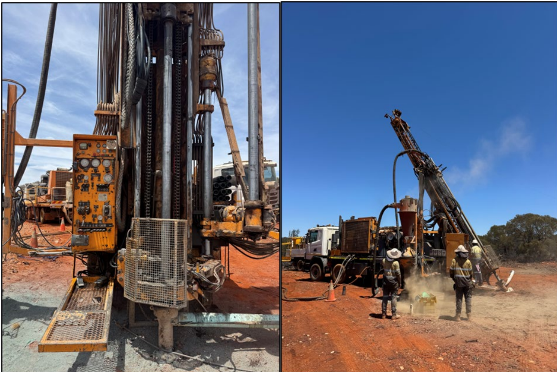
Figures 4-5: RC drilling rig in operation at the Goodenough Gold, East Menzies Gold Project, WA.
