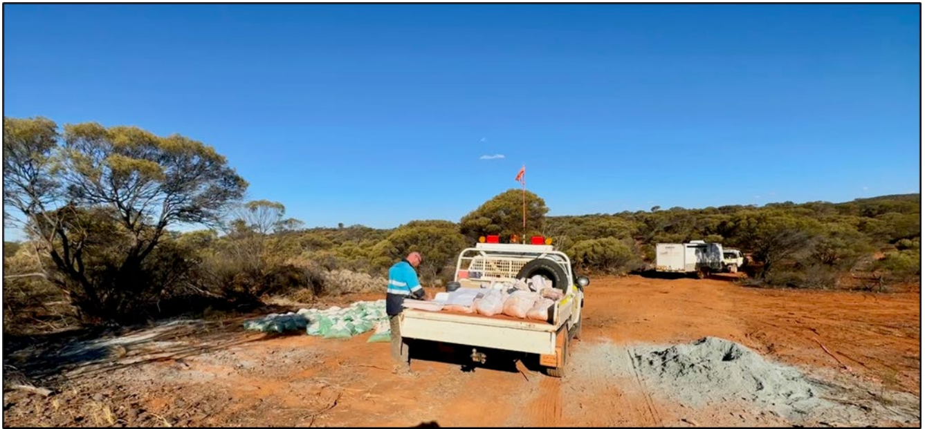
Figure 6: RC samples from drilling at the Goodenough Gold Deposit ready for dispatch.
