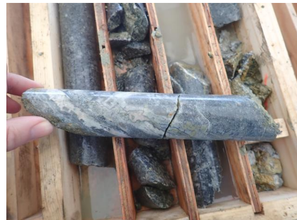
Multi-phase epithermal quartz vein, LQDD003
