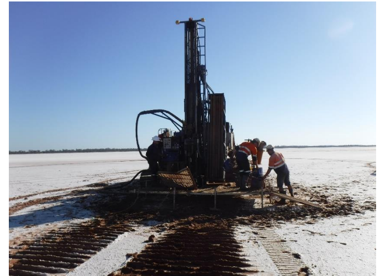
Aircore drilling on Lake Yindarlgooda, Jan 2019
