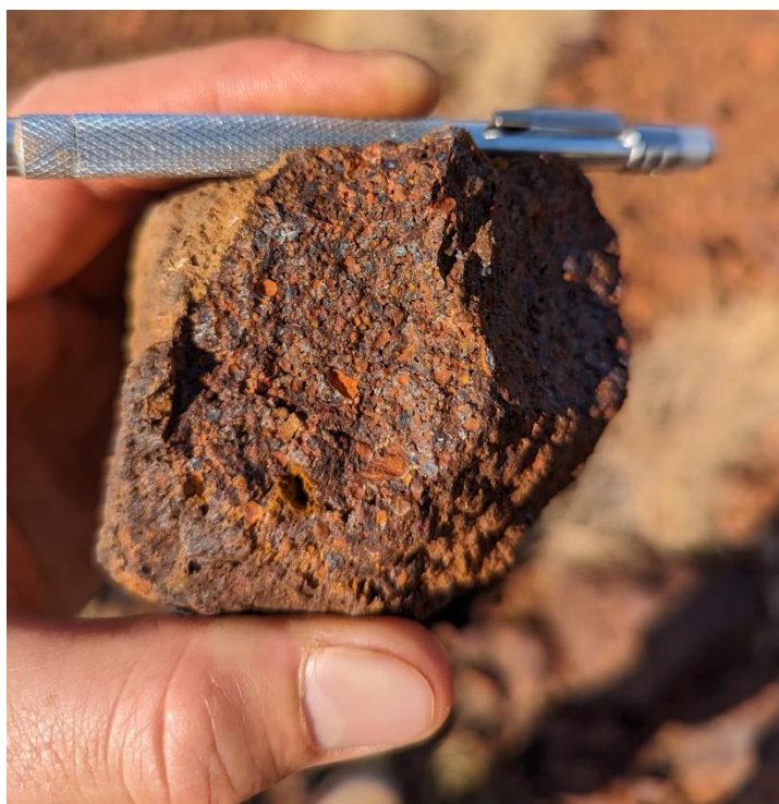
Figure 16: Robe River pisolite hand sample located from Mesa 3 (200m west of tenement boundary) showing representative Robe River pisolite found on Mesa 1 and Mesa 2
