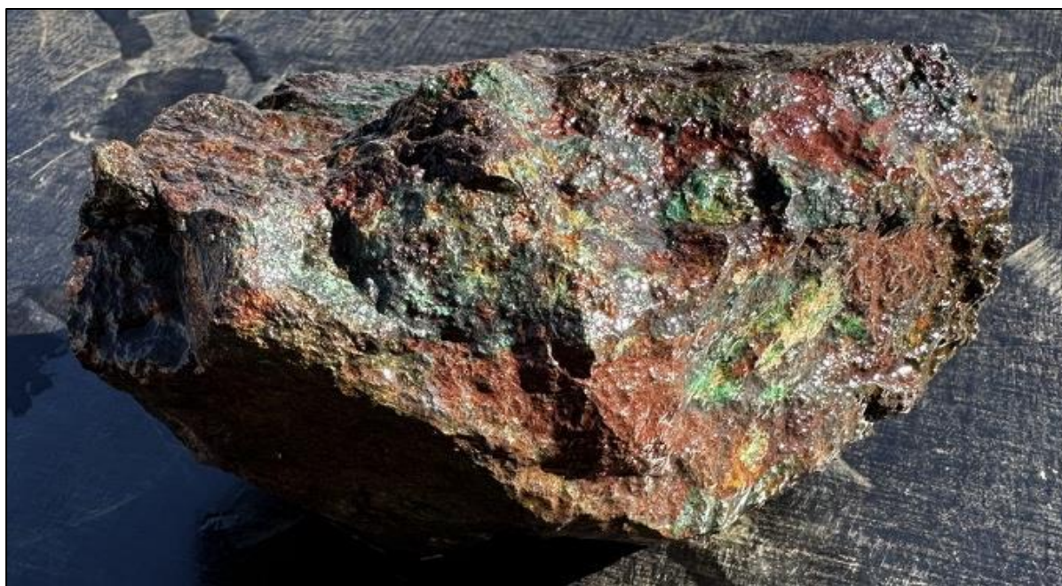
Figure 10: Hawkstone Prospect sample TEM11 that assayed 21.78% Cu and 3.3 g/t Au
