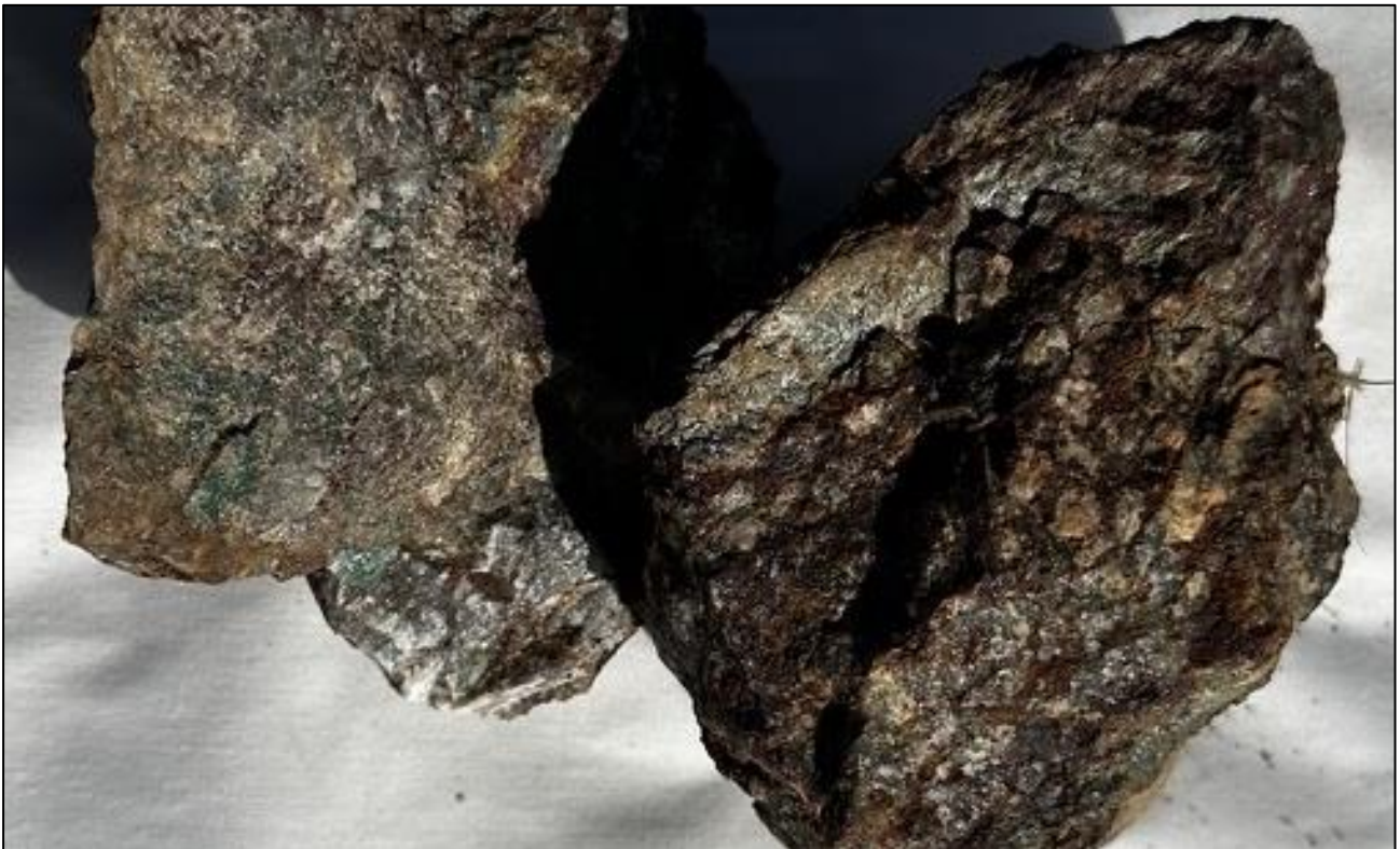
Figure 12: Lone Star Prospect sample TEM15 that assayed 4.11% Cu and 82.2 - 101 g/t Au (101 g/t Au = 3.2 Oz/t Au)
