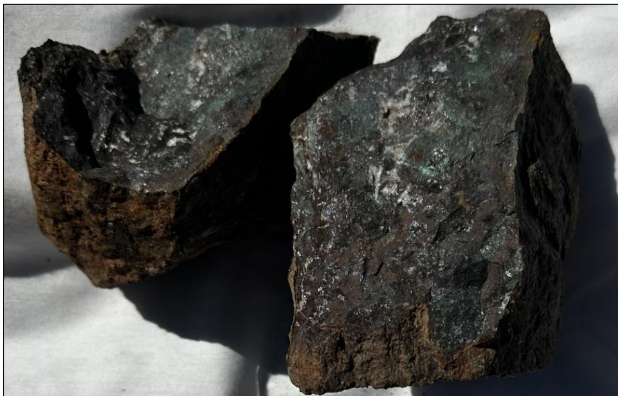
Figure 13: Hawkstone Prospect sample TEM01 that assayed 16.78% Cu and 2.4 g/t Au
