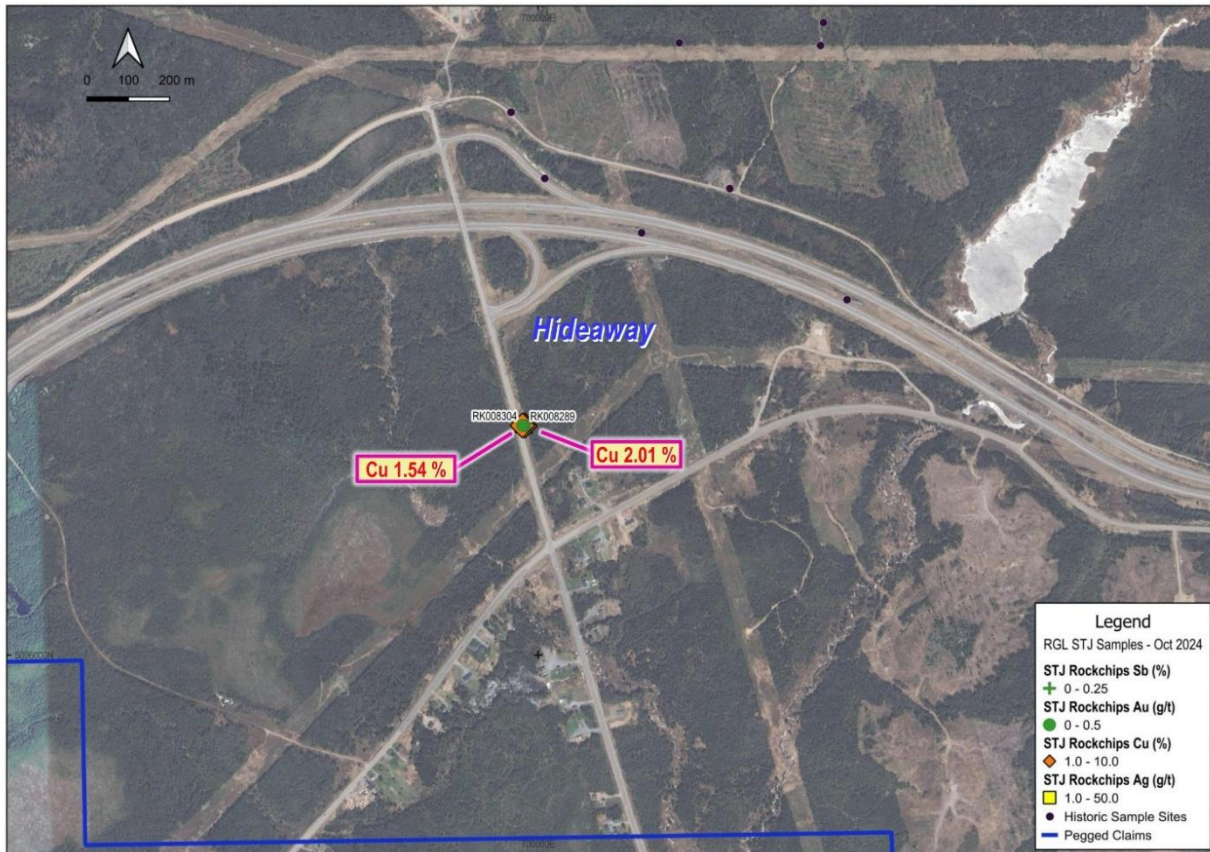
Figure 4: Hideaway prospect location showing RGL rock chip sampling locations and highlighting significant multi-element results.
