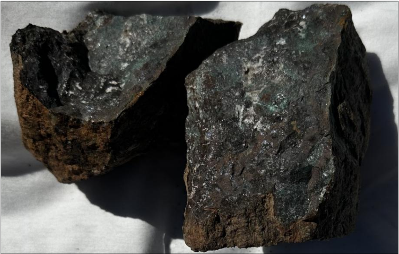
Figure 14: Hawkstone Prospect sample TEM01 that assayed 16.78% Cu and 2.4 g/t Au 11
