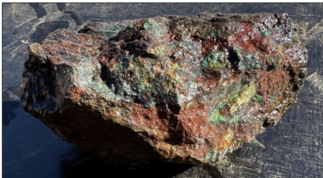
Figure 11: Hawkstone Prospect sample TEM11 that assayed 21.78% Cu and 3.3 g/t Au 8
