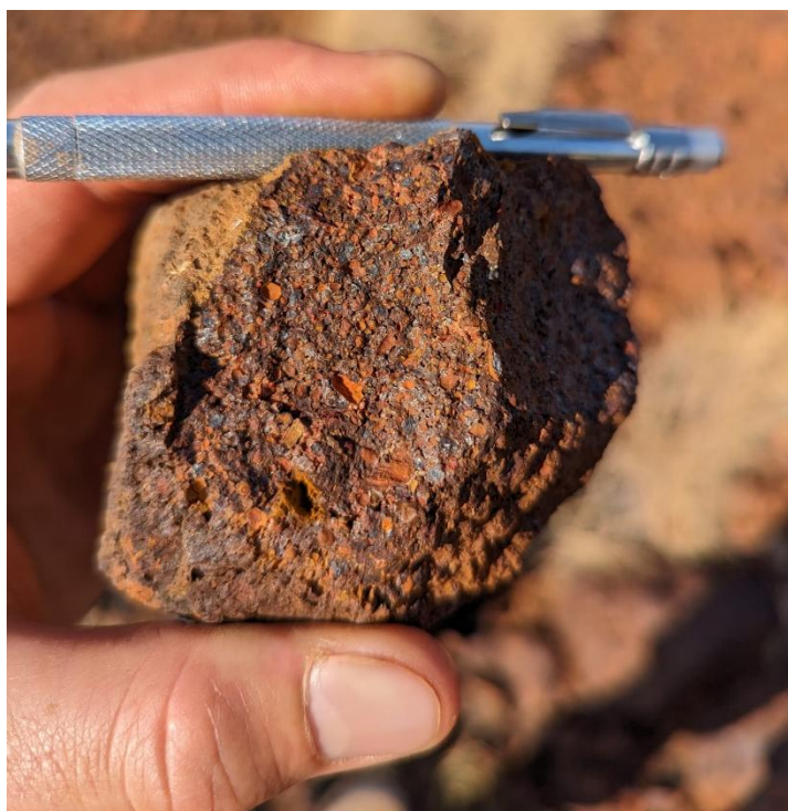
Figure 17: Robe River pisolite hand sample located from Mesa 3 (200m west of tenement boundary) showing representative Robe River pisolite found on Mesa 1 and Mesa 2
