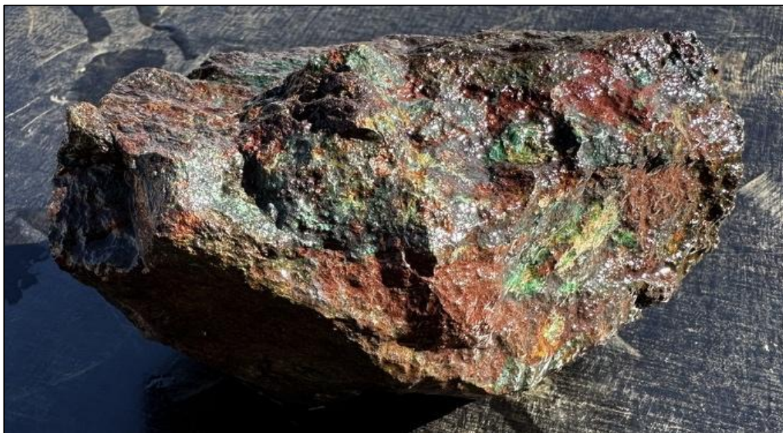
Figure 13: Hawkstone Prospect sample TEM11 that assayed 21.78% Cu and 3.3 g/t Au 14
