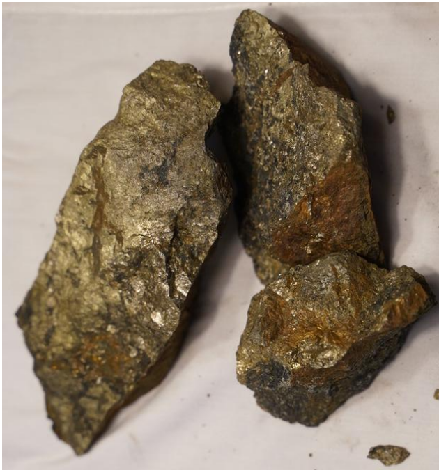
Figure 10: Prince Of Wales prospect sample RK008302 10.15% Cu and 65.8g/t Ag 11 , being tested for Induced Polarisation, chargeability, galvanic resistivity and inductive conductivity
