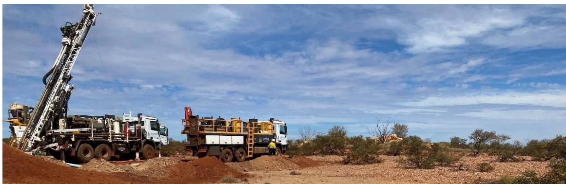
Figure 1: RC Drilling at S-Bend
