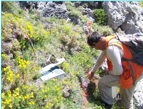
Figure 3– Ground IP Surveys can be very effective in identifying non-outcropping minerals deposits
