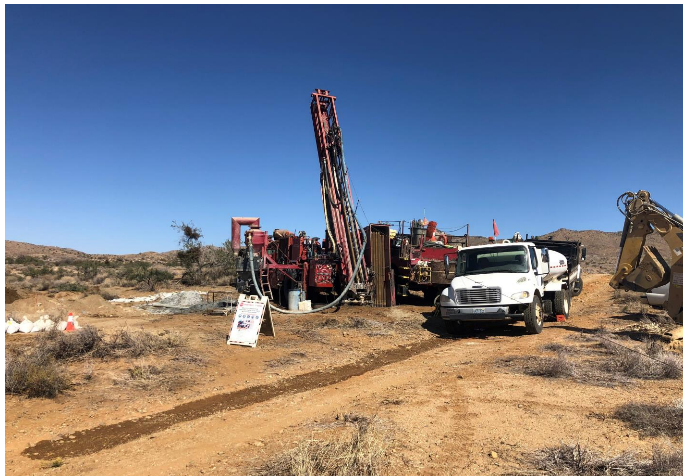
RC Drilling – October 2021
