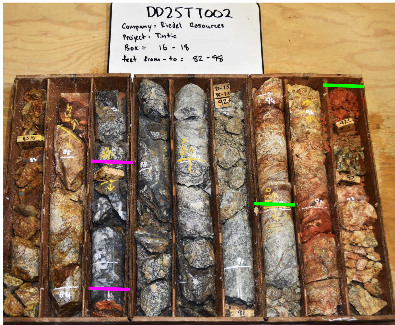
Figure 2: Mineralised zone in DD25TT002 which contains 0.91m @ 3 g/t Au, 7 g/t Ag from 22.71m (highlighted magenta) and 1.52m @ 1.54 g/t Au, 4.74 g/t Ag from 28.35m (highlighted green).
