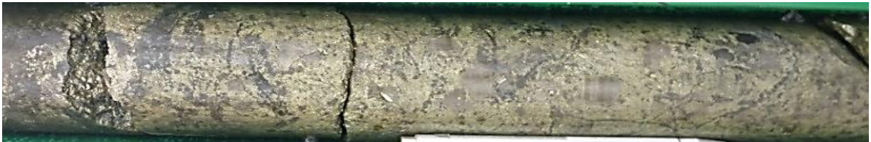
Core at 190.8m: Massive chalcopyrite-pyrite replacement in matrix of breccia
