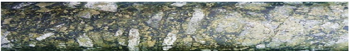
Core at 188.5m: Chalcopyrite-pyrite-tourmaline matrix of breccia
