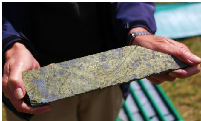
Section of core containing massive chalcopyrite at 190m in CH-DDH012. The chalcopyrite occurs in the matrix of the breccia.
