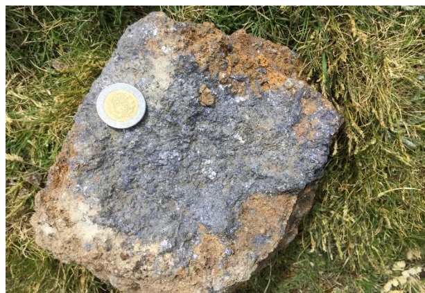
Figure 11: ABOVE LEFT Rock sample from the Torrepata Mine showing secondary zinc mineralisation (possibly smithsonite). ABOVE RIGHT Rock sample of the principal vein mined at Torrepata Mine showing zinc and lead sulphides.
