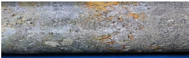
Figure 2: LEFT Core photo at 97.3m in CH-DDH018. The grade of the corresponding 97m-98m sample is 3.41g/t Au, 26.0g/t Ag and 0.31% Cu.
