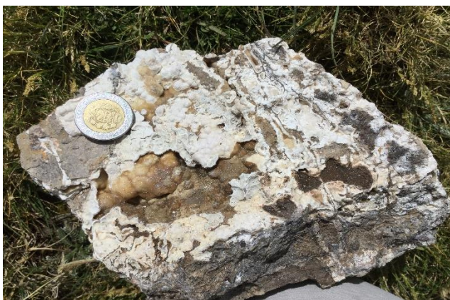
Figure 11: ABOVE LEFT Rock sample from the Torrepata Mine showing secondary zinc mineralisation (possibly smithsonite). ABOVE RIGHT Rock sample of the principal vein mined at Torrepata Mine showing zinc and lead sulphides.
