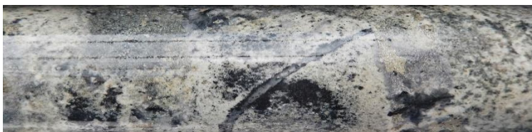
Figure 7: LEFT Core photo at 581m (CH-DDH027) Veined and highly altered monzodiorite with multiple forms of sulphide.
