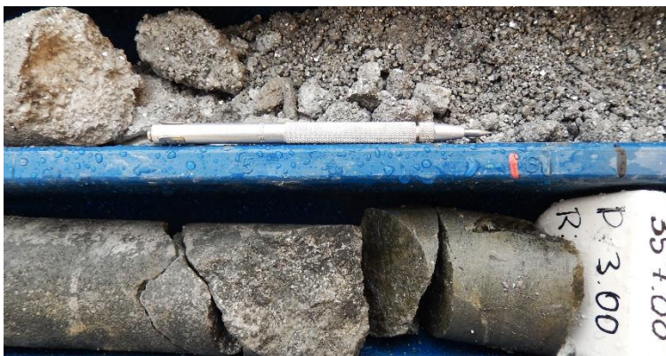
Figure 4: LEFT Core photo at 357m (CH-DDH027): Massive to semi-massive sulphide zone.
