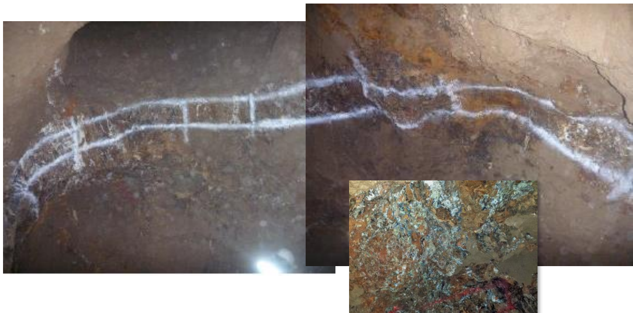
Figure 2: BELOW Photo mosaic of Channel 4 (C4). C4 corresponds to the intersection of the new NS vein and HV-02. This 5.7m long channel sample has an average grade of 1.72% Zn, 74.4g/t Ag, 6.02% Pb (Table 1) with peaks of 5.74% Zn, 162.0g/t Ag, 11.75% Pb . INSERT: Detail showing the semi-gossanous nature of the vein. It is thought grade values, particularly of Zn, may improve as weathering decreases at depth.
