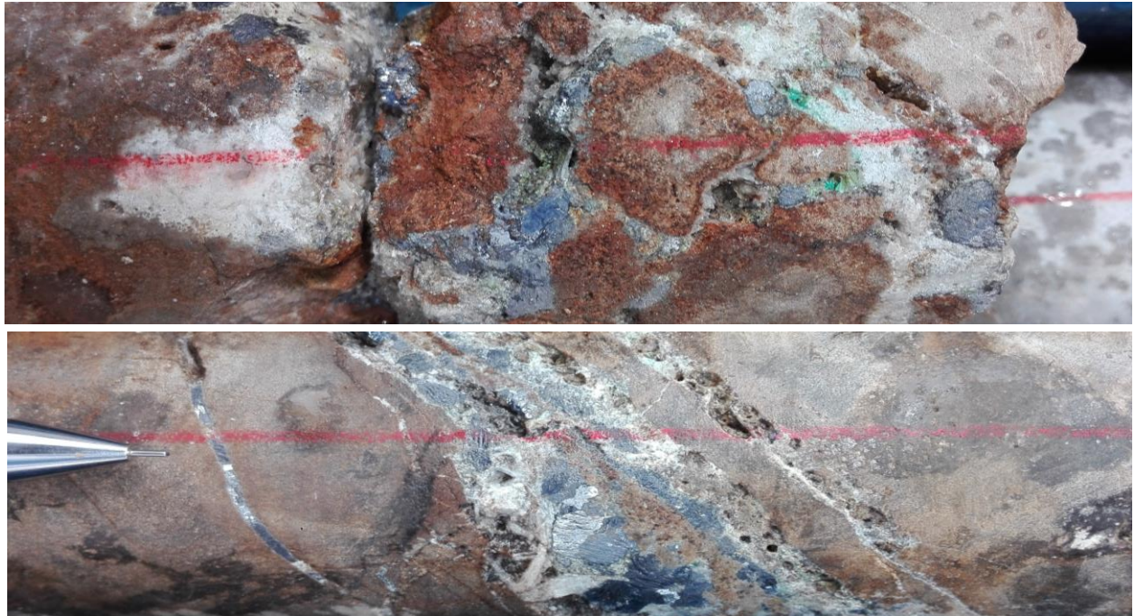
Figure 5: ABOVE Core photos of possible manto between 22.85m and 25.85m depth in RDDH-019. ABOVE TOP The manto is brecciated and shows signs of secondary copper (Cu) mineralisation (green mineral in matrix). The sample corresponding to this core photo grades 1.87% Zn, 138g/t Ag and 7.1% Pb . ABOVE BOTTOM Mineralised veinlets parallel to limestone bedding. Coarse galena (Pb sulphide) and smithsonite (Zn carbonate) occur within the veinlets.
