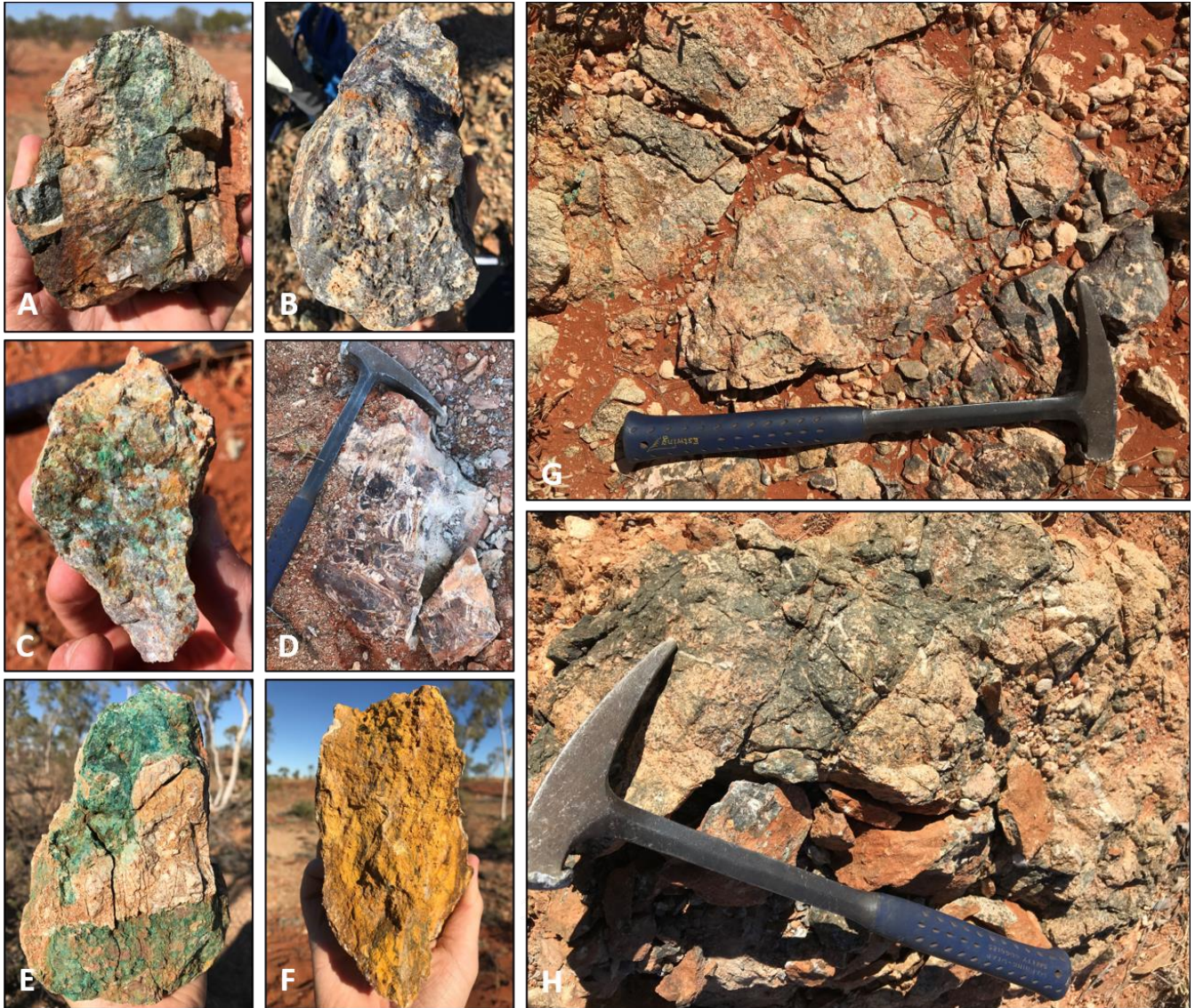
Figure 4 Selection of Ningaloo rock chips including: A) JE0094 with 0.36g/t Au + 1.42% Cu + 957ppm Bi; B) JE0105 with 0.19% Cu; C) JE0098 with 1.27% Cu; D) JE0103 with 0.46% Cu; E) JE0107 with 9.65% Cu + 2.93g/t Ag; F) JE0108 with 0.16% Cu; G) JE0096 with 1.28% Cu; and H) JE0110 with 0.19% Cu.
