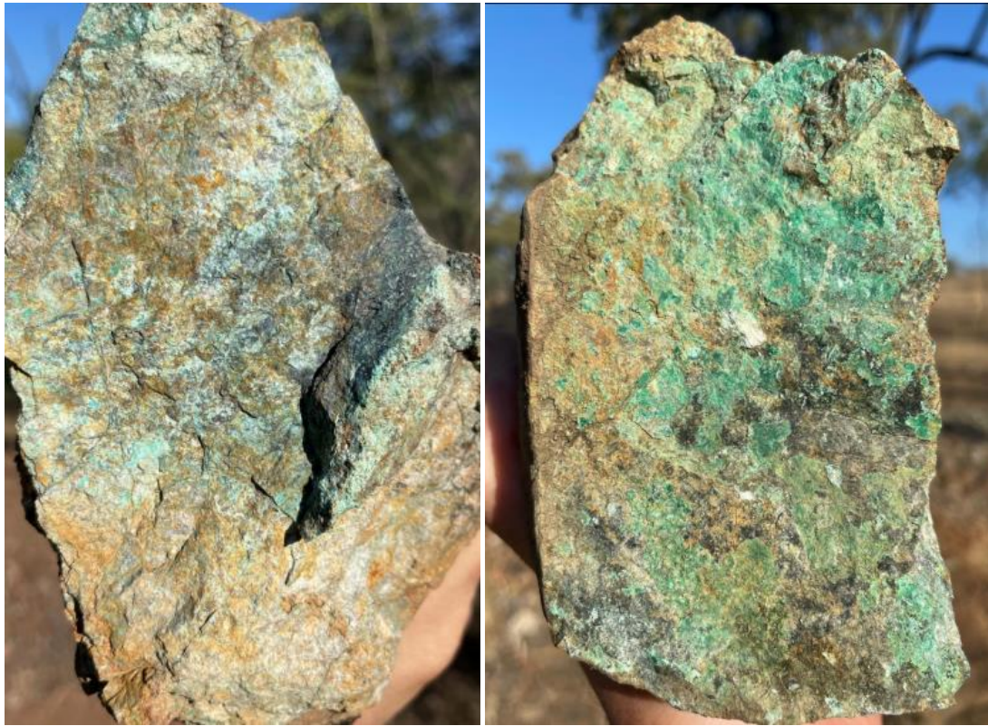
Figure 10: Sample photos. MC0088 (left) Malachite-azurite bearing granite with quartz veining. MC0093 (right) Quartz-malachite lode (15m wide) collected from a mine working.
