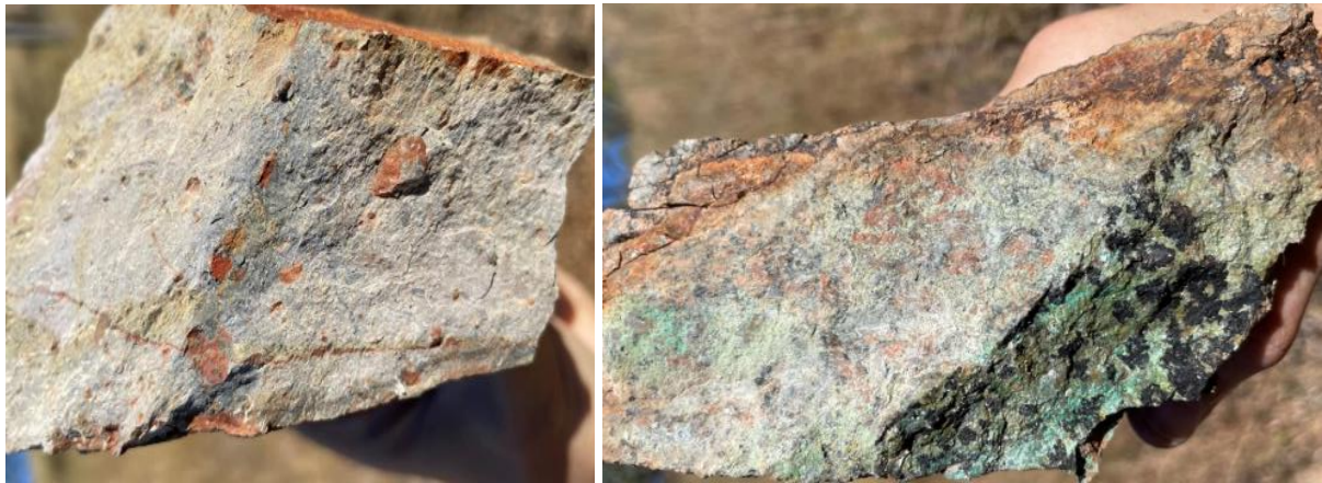
Figure 8: Sample photos. MC0077 (left) Bleached andesite. MC0080 (right) Malachite-chrysocolla bearing quartz vein mineralisation.
