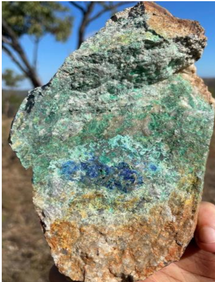
Figure 14: Sample photos. MC0166 (left) Malachite-azurite bearing intrusive rock.
