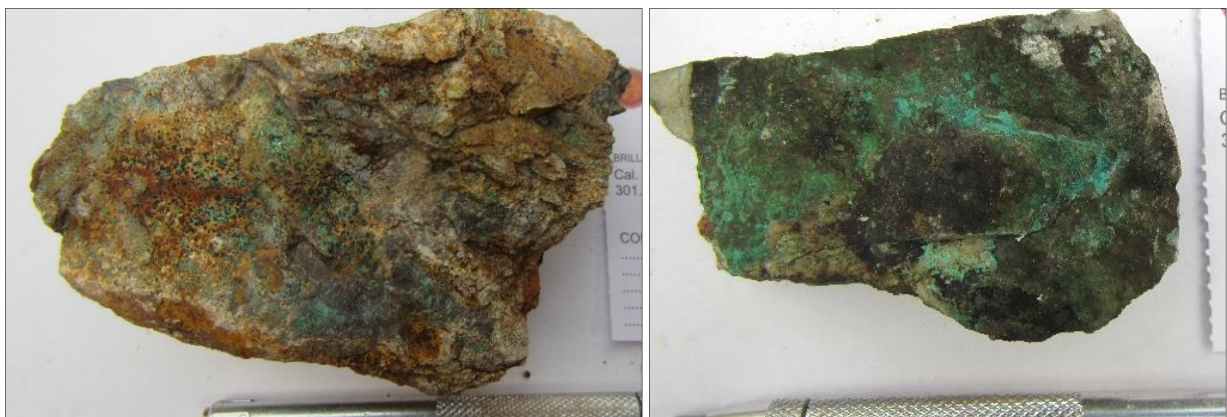
Figure 8: Sample photo of BM-01377 (left) and BM-01366 (right). Sample BM-01377 contains 2.98% Cu and Sample BM-01366 contains 2.92% Cu. The samples are of mineralised breccias that contain secondary copper minerals.
