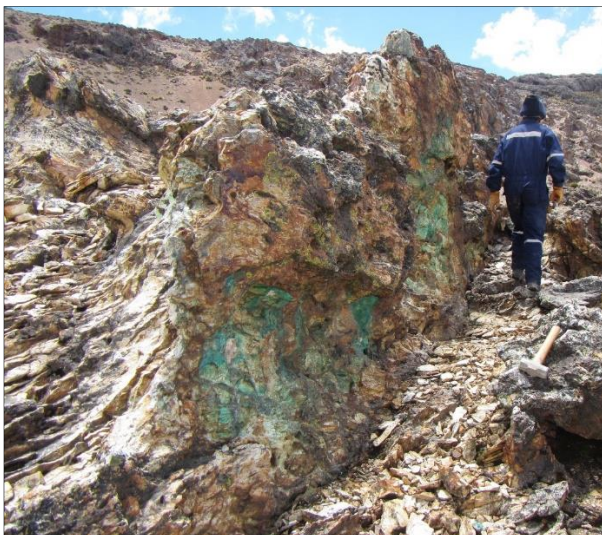
Figure 6: Outcrop photo showing extensive massive secondary copper mineralisation (malachite and chrysocolla) located on the new Occorccocho II concession. This photo first appeared in ASX announcement dated 16 August 2021. Sample photo of BM-01185 (right). BM-01185 taken from this outcrop contains 1.95% Cu and 197g/t Ag.
