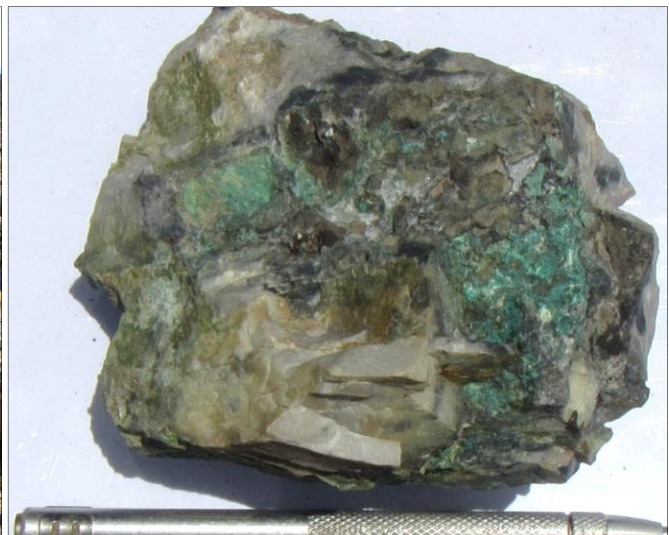
Figure 6: Outcrop photo showing extensive massive secondary copper mineralisation (malachite and chrysocolla) located on the new Occorccocho II concession. This photo first appeared in ASX announcement dated 16 August 2021. Sample photo of BM-01185 (right). BM-01185 taken from this outcrop contains 1.95% Cu and 197g/t Ag.
