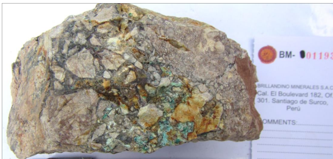
Figure 1: Photo of sample BM-01193 which contains 2,238g/t Ag (the highest Ag value to date at greater Riqueza) . It is a brecciated and highly altered volcanic with visible copper mineralisation. As well as bonanza grade silver, the sample contains 0.15% copper and 0.66% lead.
