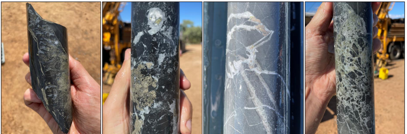
Figure 3: Core photos taken rig-side at FW220006. Left: Pyrite-quartz veining in graphitic schist at 648m. Localised pyrite content is between 10-30%. Centre Left: Chalcopyrite-carbonate and quartz-pyrite-carbonate veining in graphitic schist at 685m. Localised pyrite content is between 10-20%. Localised chalcopyrite content generally <1% to trace. Centre Right: Pyrrhotite-chalcopyrite-quartz-carbonate veining in dolomitised metasiltstone at 723m. Localised pyrrhotite content is between 10-20%. Localised chalcopyrite content generally rare to trace. Right: Quartz-carbonate-dolomite breccia zone within metasiltstone at 679m.
