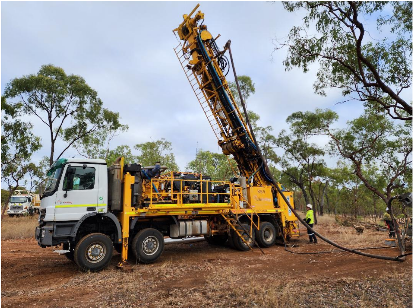
Figure 1: The multi-purpose DE840 rig currently drilling onsite.
