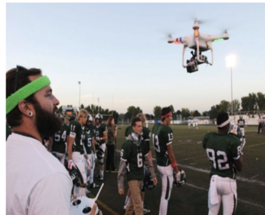
This is the first ever FAA waiver for UAS flight over people with a parachute safety system.
