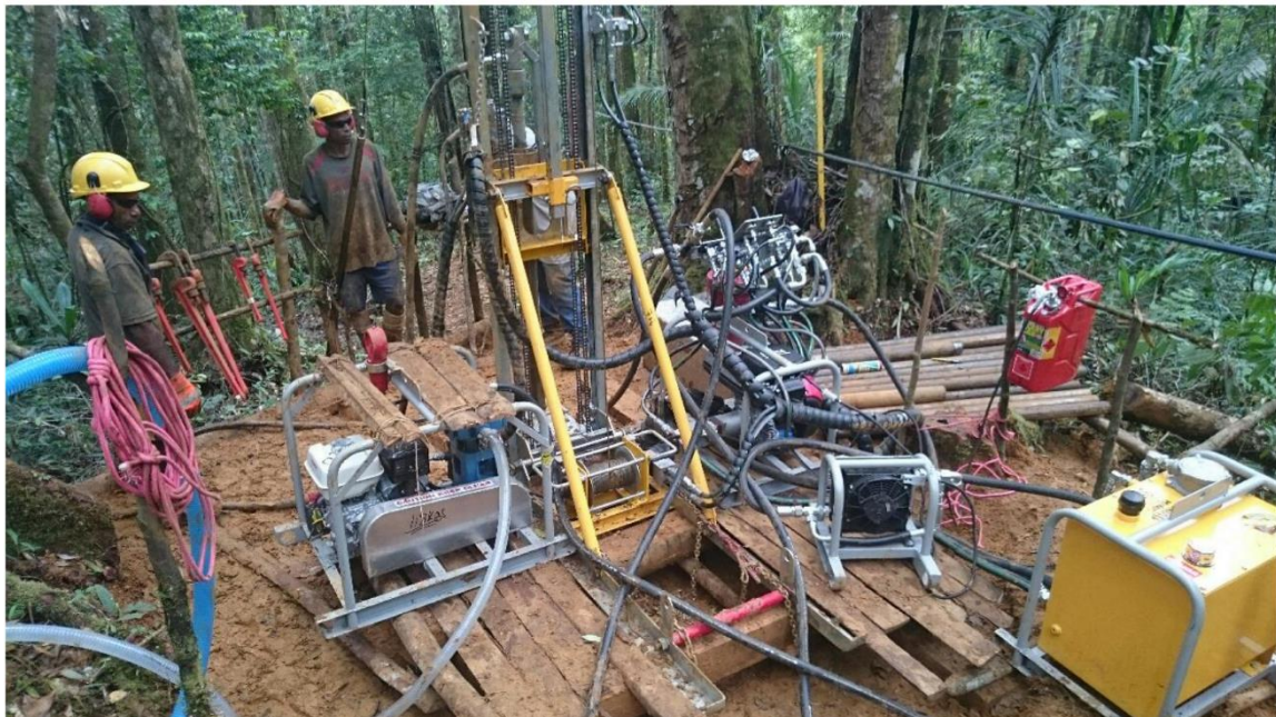
Figure 10 - Man portable diamond rig used for the 2015 drilling campaign.
