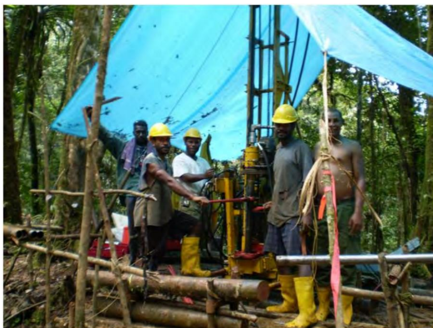
Figure 15 - Man portable rig used by Paradise Drilling Pty Ltd for 2007-2008 program
