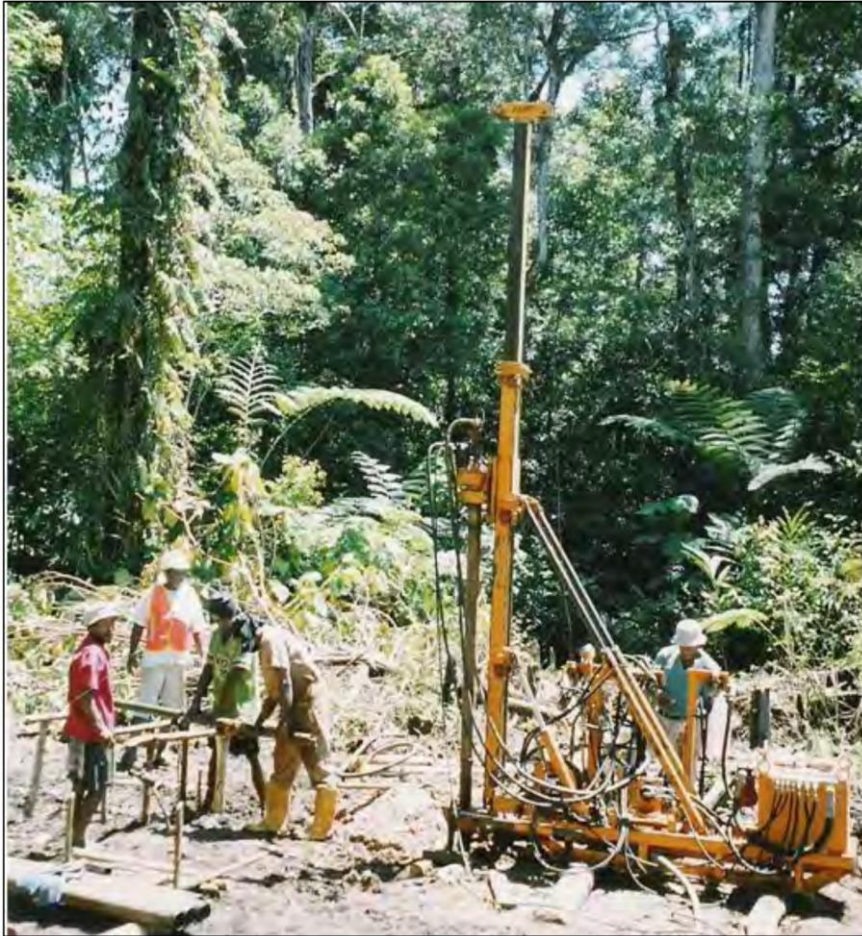
Figure 14 - Man portable diamond rig used for HQ core during 2003-2004 drilling campaigns
