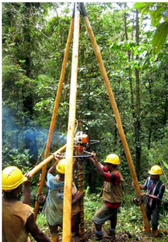
Figure 16 - Niugini Nickel man portable rotary auger core rig 2011
