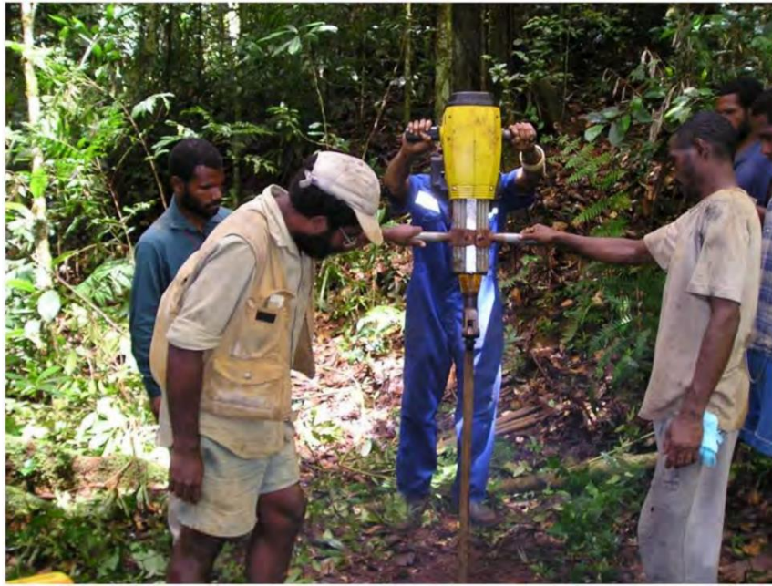
Figure 13 - Wacker rig used for core drilling in 1999, 2004, 2008 programs.
