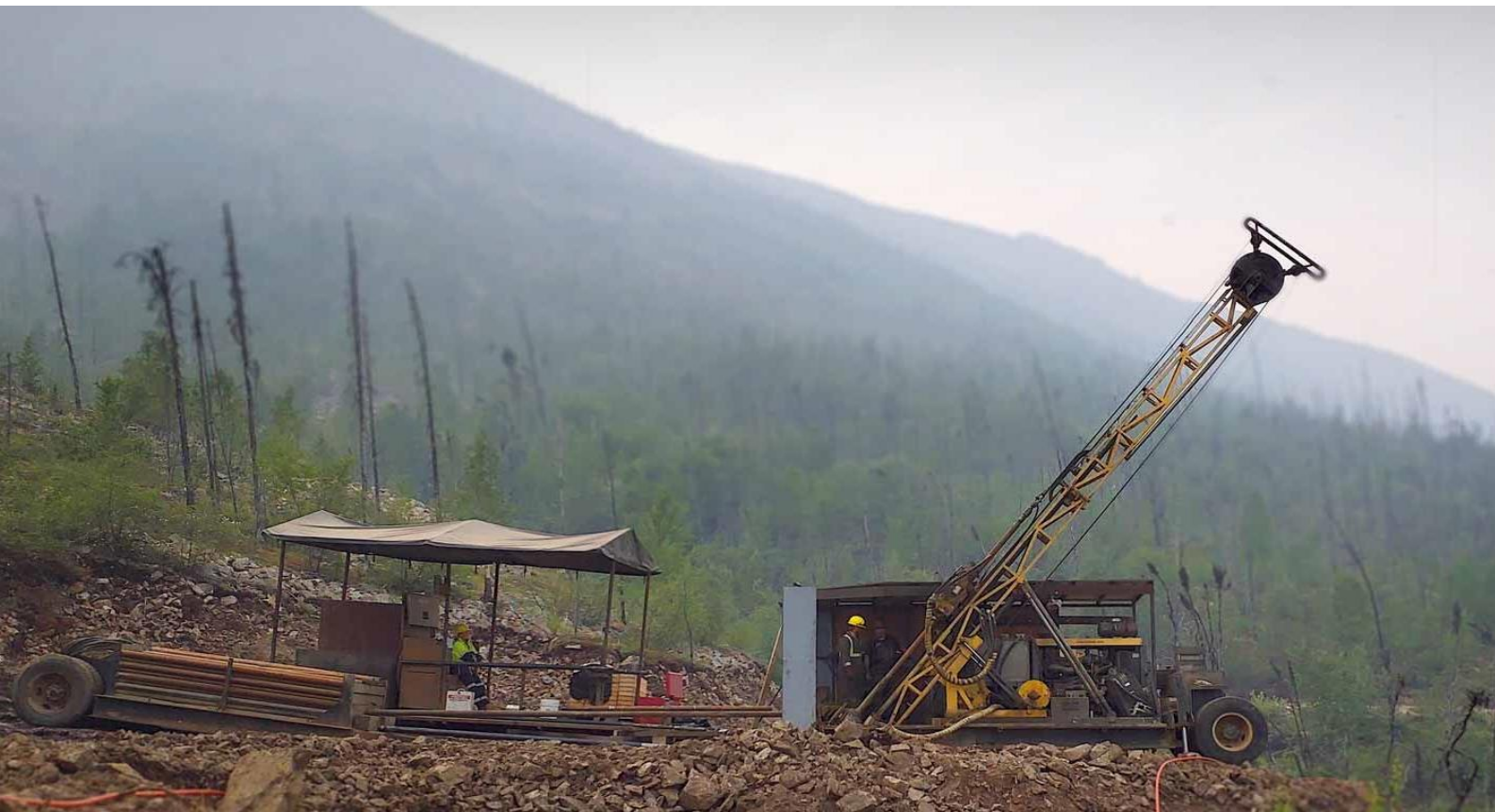
Figure 1 Drilling (Diamond Core Rig) on the 64North Project (June 2022.)
