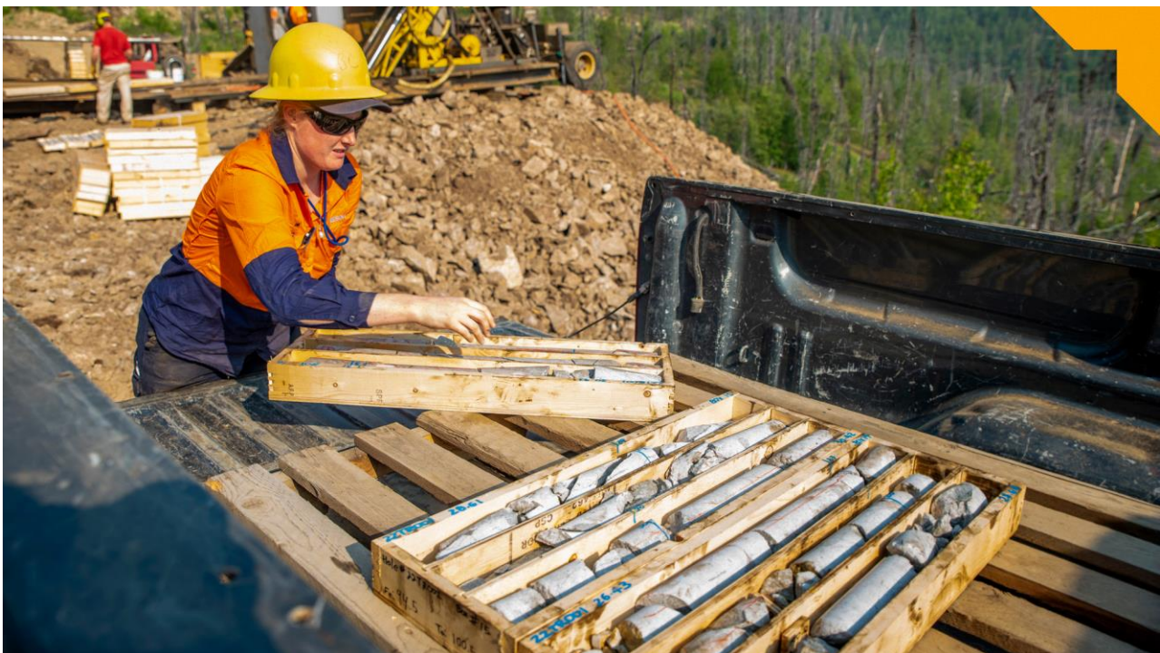
RML team getting core samples ready for transport for logging and sample preparation.
