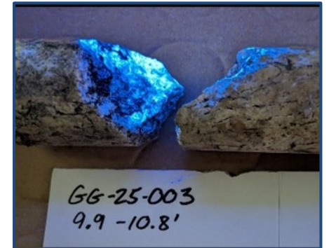
Photo of drill core HHGG25-003 (9.9ft to 10.8 ft downhole depth) showing an oxidised manganese-quartz mineralised vein cross-cutting altered quartz-feldspar intrusive, with 2% scheelite estimated of core section. Source: ASX announcement 8 Sept 2025.
