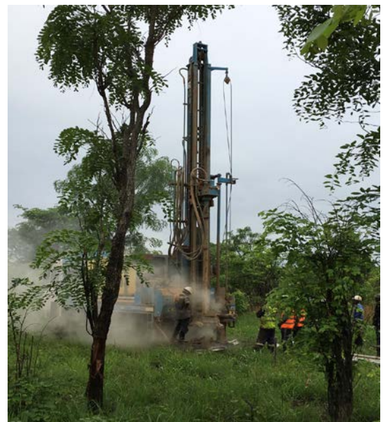
Figure 1: A: Sampling team including geologist and helpers collecting soil samples. B: RAB/AC drill rig completing drill hole on the palaeochannel grid.
