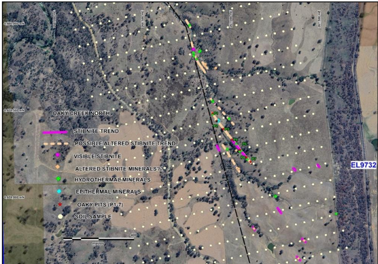
Figure 14: Initial field interpretation and sampling of the Oaky Creek North area to be validated with assay results. Note some of the samples are float, so those samples on soil traverses may not be insitu.
