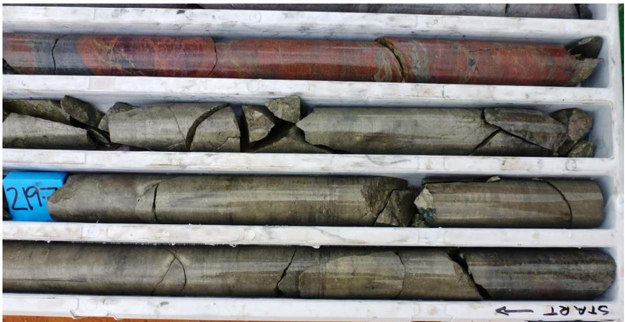
Figure 3. Hole EEDD012 – portion of massive sulphide interval from 217.5 metres to 221.5 metres
