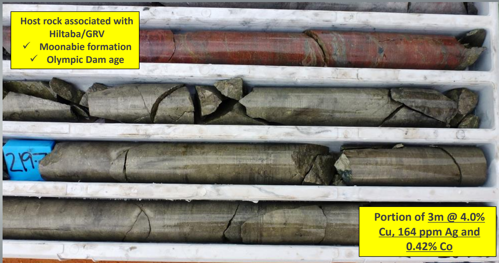
Hole EEDD012 – portion of massive sulphide interval from 217.5 metres to 221.5 metres
