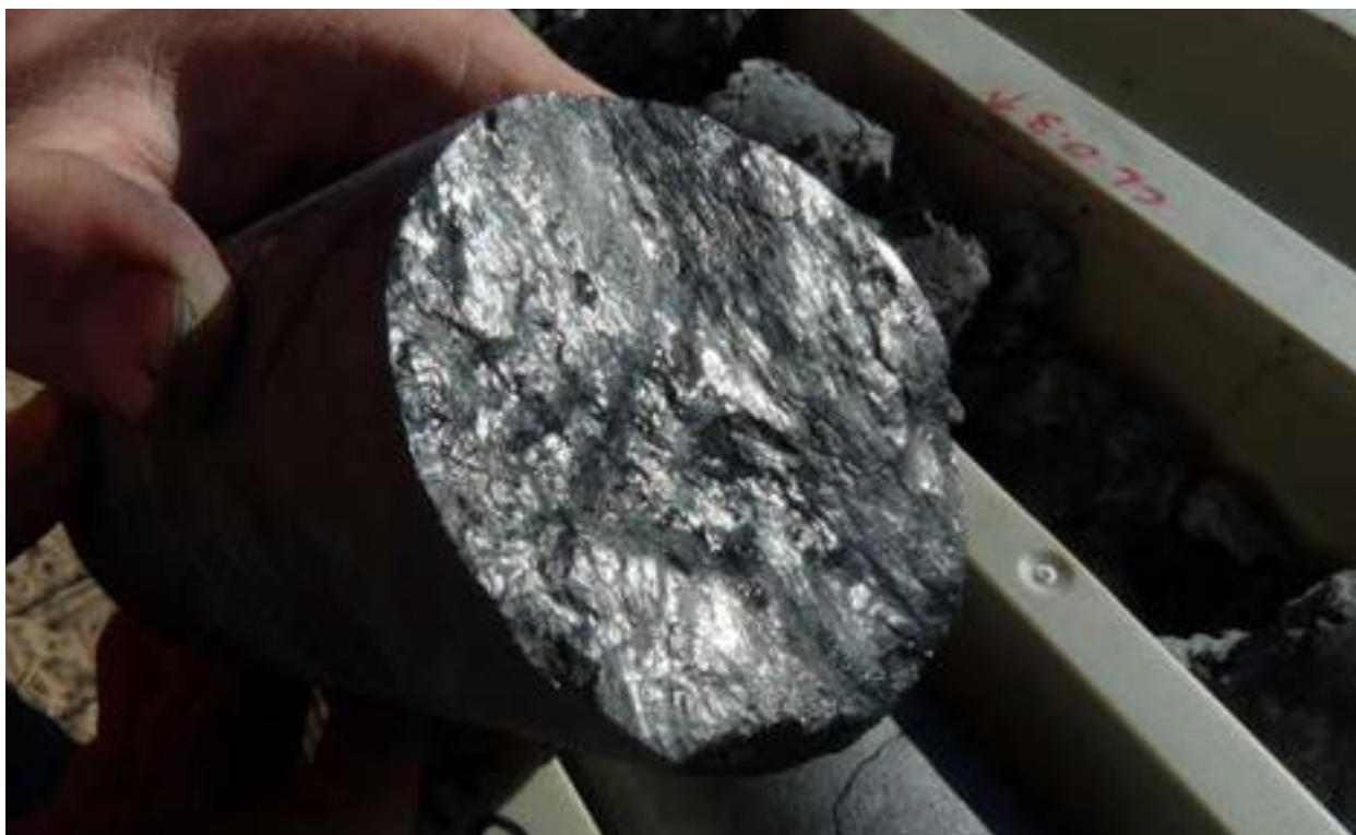
Figure 1. Diamond core drill sample showing graphitic intersection at Siviour prospect (SIVD007, 52.6m to 53.5m @ 9.3% TGC)
