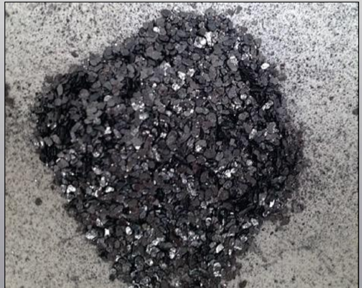
Extra large coarse flakes ( \gg 600\mu m) from diamond core hole (CRD090) at Siviour prospect
