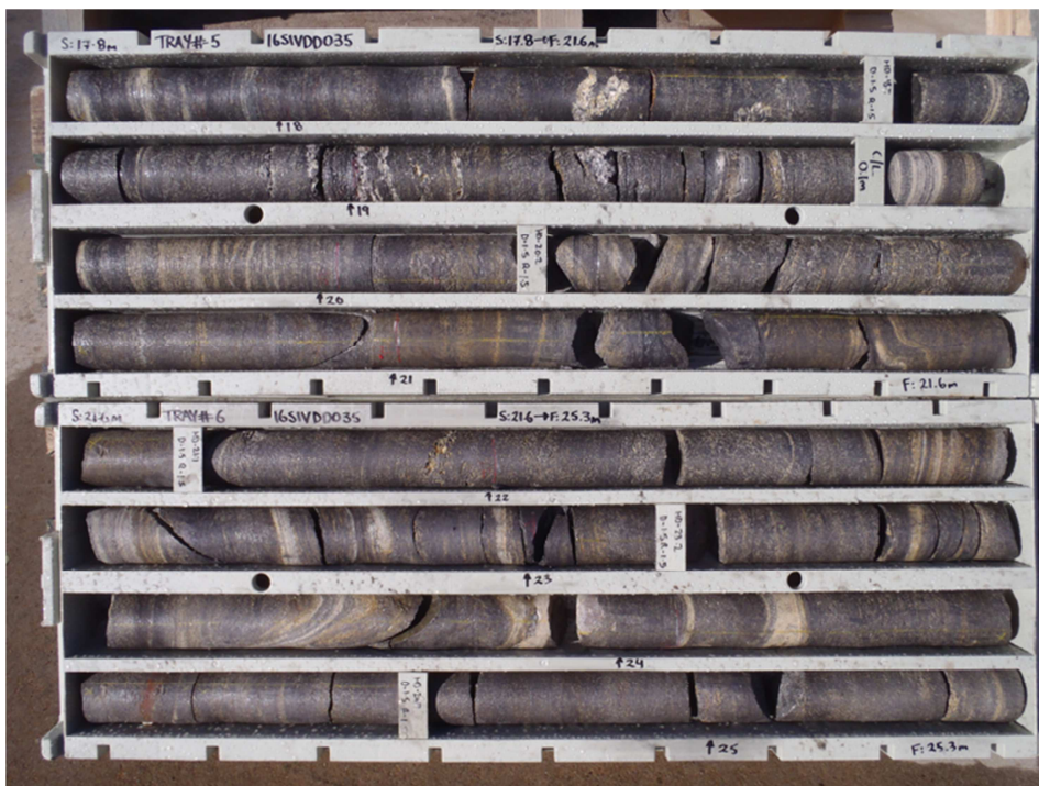
Figure 1. Diamond core drill sample showing graphitic intersections at Siviour Graphite Deposit (SIV035 -- 17.8m to 25.3m, including 7m@ 15.8% TGC)
