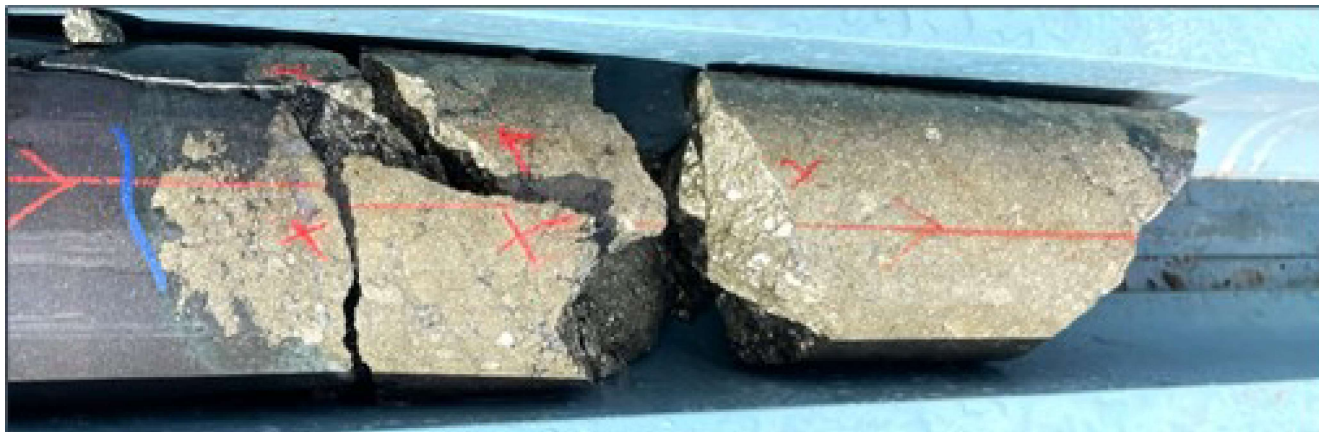
Figure 4. RMD001 massive pyrite, at 212m down hole.
