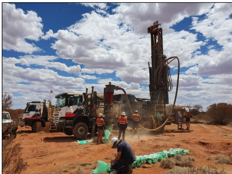
Image 1 – RC Drilling rig operating at Earraheedy Project
