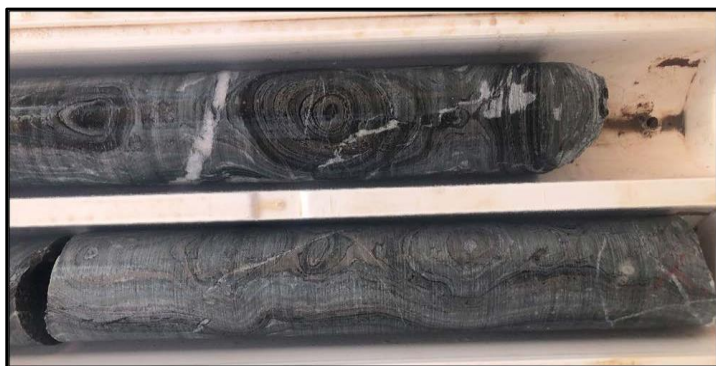
Image: NQ2 core from diamond drillhole 20ALD0006 showing basin and dome interference patterns in tightly folded quartz sandstones. Similar folding is well documented at Telfer and is considered to be a major control on the distribution of gold and copper mineralisation within the Telfer orebodies.
