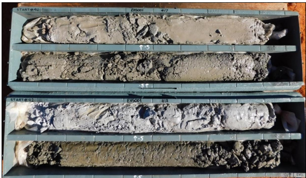
Figure 2 – Mineralisation Zone –Sonic Drilling Core – EHS001 (twin of EHR050). Sphalerite, galena and pyrite mineralisation was logged in this soft primary zone.
