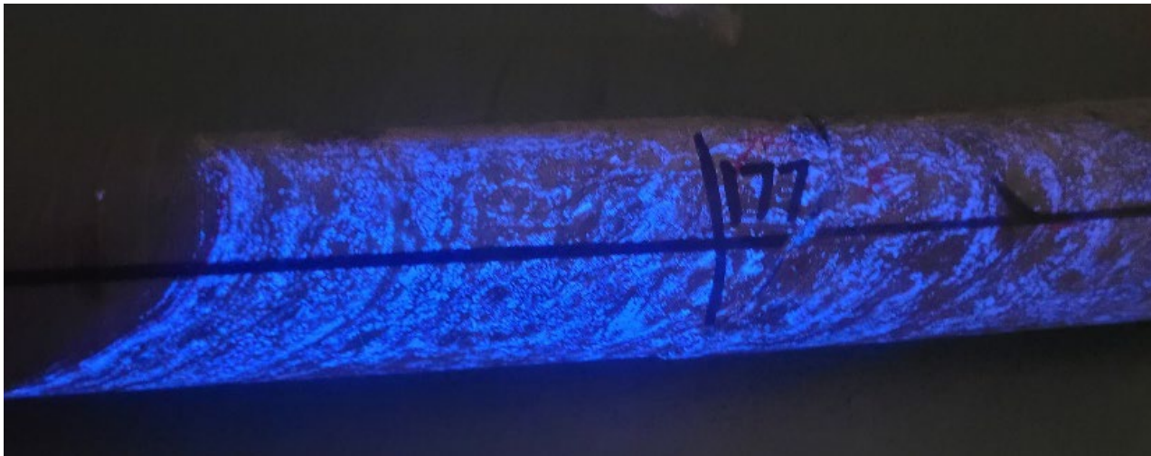
Figure 5 - WQDD013 (0.65m @ 18.35 WO 3 ) scheelite intersection under UV light
