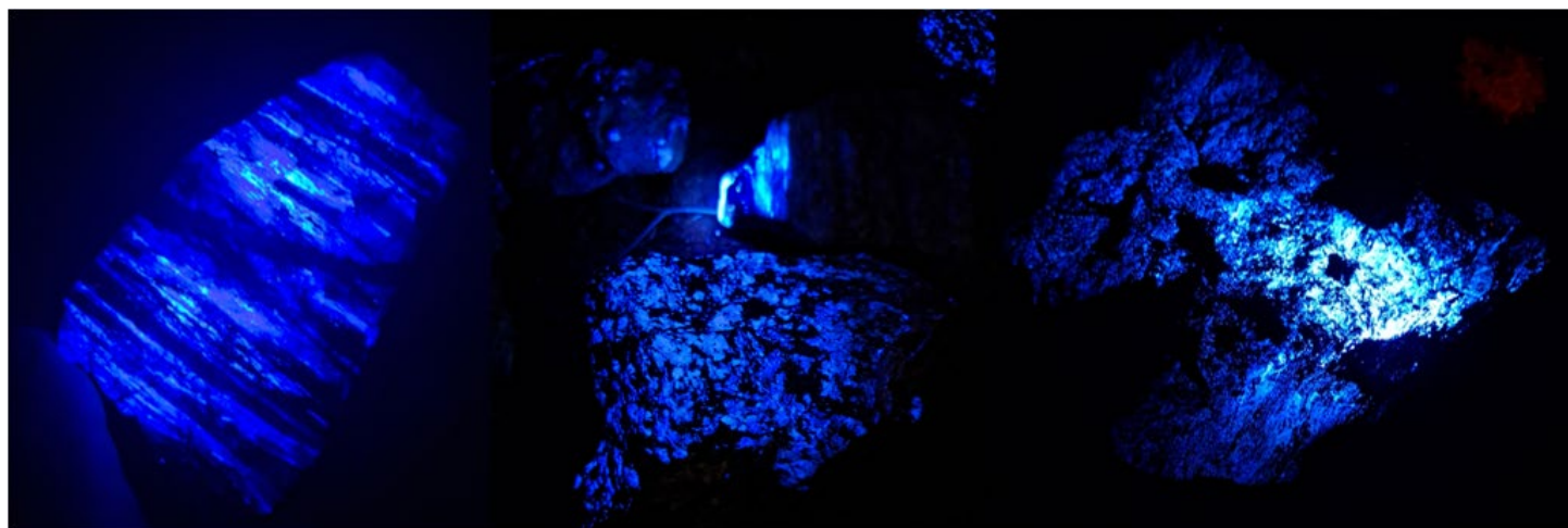
Figure 4 - Examples of scheelite bearing samples identified by UV light in containment bunds and on waste rock dumps at Western Queen. Note: samples shown are not to scale.
