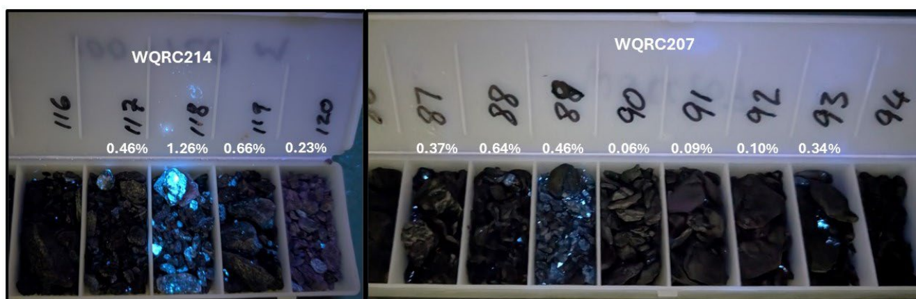
Figure 3 – WQRC214 (left) and WQRC207 (right) chip trays under UV light demonstrating the relationship between scheelite mineralisation in chips and their associated tungsten (WO 3 %) laboratory assays
