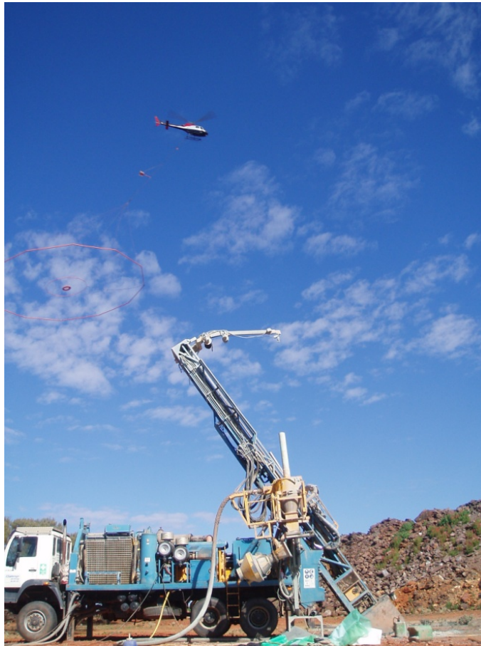
VTEM (helicopter and hanging EM loop) being flown above RC drilling rig at Mt Fisher
